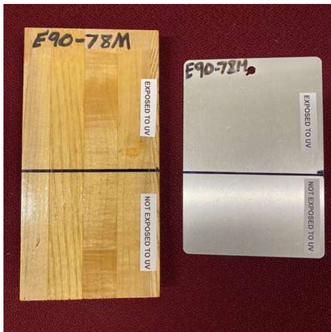
Figure 3: wood and aluminum panel samples coated with KEY Tough-Coat E90-78
